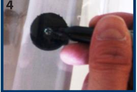
4. Place your cover over the well. Use a marker to mark the location of the Dual-Lock<sup>™</sup> disc. You will use this mark to attach the corresponding Dual-Lock<sup>™</sup> pad to the underside of your cover. Clean the area under the cover before you adhere the Dual-Lock<sup>™</sup> Pads
