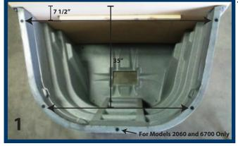
2. Models 2060 and 6700: Measure out from the foundation 7 1/2" and place a mark on both sides of the well. Then measure out 35" from the foundation and mark the location. The final Dual-Lock<sup>™</sup>disc will be placed at the center front of the well (As Shown to Above)
