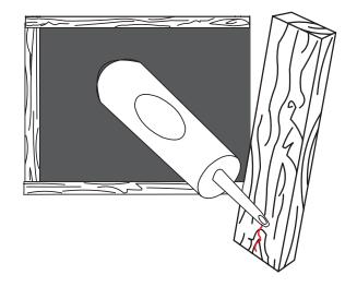
Anchor locations. Fasten into concrete opening with concrete fasteners.
