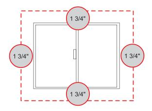
Cut and remove the piece out of the wall.
