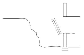
Using womanized lumber, build a frame for the window to sit in. Secure the wood using silicone. Once silicone is dry use concrete fasteners to secure lumber properly.
