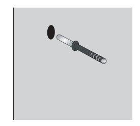
Line up the top mounting hole with the expansion bolt, and hang well on wall. While still holding the well, making sure that the expansion bolt has slid securely into place, use a level to mark the placement of the other bolts on the wall.
