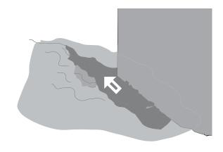
Whether using a contractor or cutting the hole yourself, outline a square on the wall that is  $3\frac{1}{2}$ " bigger all the way around the window. Make sure lines are square and  $90^{\circ}$ .
