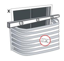
For proper mounting use the top two holes on the well and then every 10" down the well. Make sure that the bottom hole has a screw so that all four corners are securely fastened during backfill.
