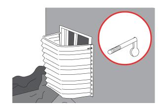
Be sure to mark the X for drilling at the top of the mounting eyelet, so that the well remains level. Remove the well after holes have been marked. Drill the X's for the mounting holes just as the first one was done. When finished, insert expansion bolts in each hole drilled and mount well using a washer and a nut.
