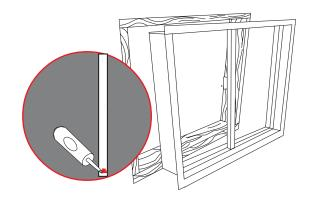
Using  $1\frac{1}{2}$ " galvanized screws, continue securing windows in wood frame using the holes provided on window frame.
