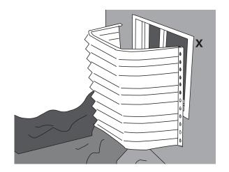
Once window is installed verify measurement of well, and mark first hole for mounting and drill hole out.
