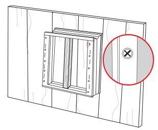
With one corner attached to the wood form, use that area to pivot the Easybuck<sup>TM</sup> frame until it is level.
