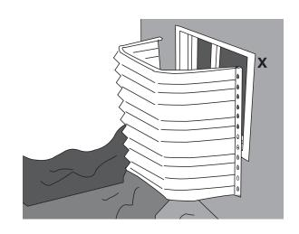
Once window is installed verify measurement of well, and mark first hole for mounting and drill hole out.
