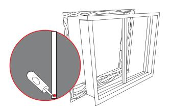
Using  $1\frac{1}{2}$ " galvanized screws, continue securing windows in wood frame using the holes provided on window frame.
