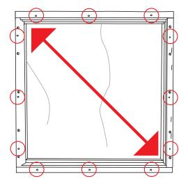
Once the second wood form is in place, locate buck in wall and nail thru from outside of wood form.
