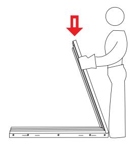
Before installing remaining Jamb, make sure that corners of the Jamb are tucked slightly to allow for overlap from Sill.
