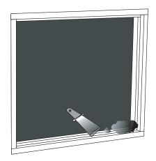
Install window from the outside. Install window over sill using fins located on bottom of window frame.
