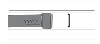
Place a small block of 2X4 wood in Jamb channel. Butt against the male tab which has been pushed through and hammer.
