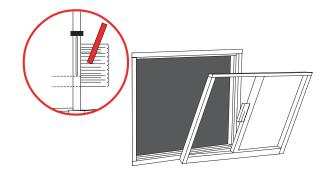
Lock window frame into place from the inside using window locking tabs.
