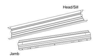
Tilt Sill at a 45 degree angle and insert end tab into Jamb slot using downward pressure.
