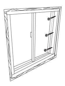
Mount well on wall allowing 12" below the window for proper drainage. Note: If drain is exposed during excavation, see drainage section for proper drain installation.
