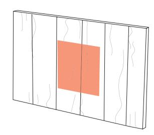
With buck screws facing out, attach one corner of buck to wood form making sure the bottom of the buck is no more than 40" from the floor for Egress. See Egress Section for complete IRC 2000 code.
