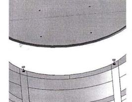
**Step 1** Acquire (4) anchor-bolts for concrete or screws/bolts for wood at least 2-1/2" long and 1/8" diameter to secure the Cover Brackets to the House Wall.
