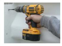
With a hammer drill and wedge drill bit, drill all pinned impression holes 23/4" deep around entire window well: sides and bottom.
